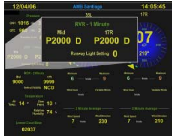
RVR and MOR as part of an integrated AWOS system
