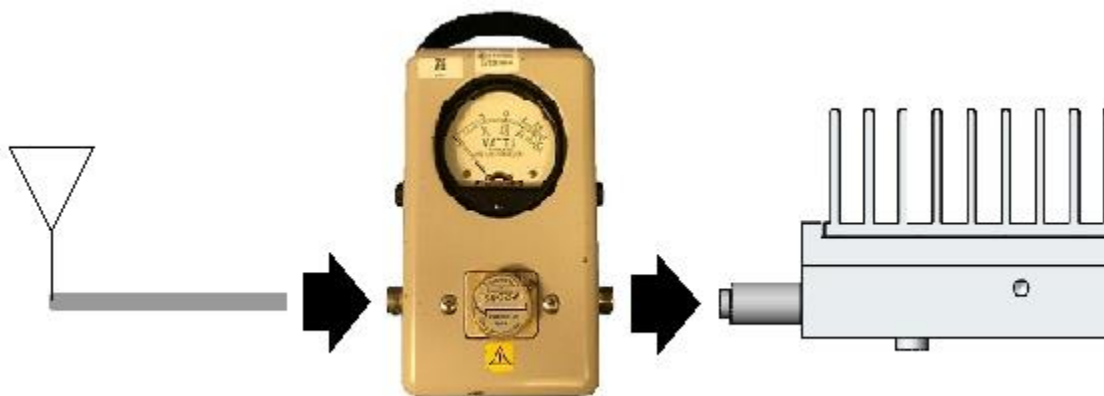
Figure 10. Insert Power Meter Between Antenna and VHF radio
