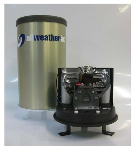
The funnel and the base heaters are controlled by thermostats; the drain tube heaters are continuous duty. Rain gauge models may operate on either 115 VAC or 230 VAC power.
