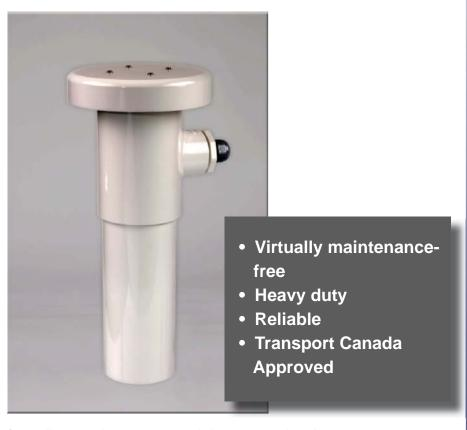
from direct moisture contact. It is constructed of heavy-duty polymer to limit thermal mass, and thereby preventing radiant heating of temperature probes by the tubing. Highly reflective white paint is applied to all exterior surfaces to reflect as much solar radiation as possible.
