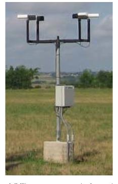
visibility measurement is not affected by contaminants on the lenses, or by temperature effects on the emitters and electronics.
