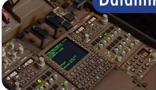
Datalink ATIS (D-ATIS) adds an additional capability to standard ATIS system. Datalink allows the pilot to receive the airport ATIS information on the aircraft ACARS message screen. This feature requires interfacing the ATIS with the air-to-ground communication provider in the region. AWI ATIS is capable of interfacing with all providers.
