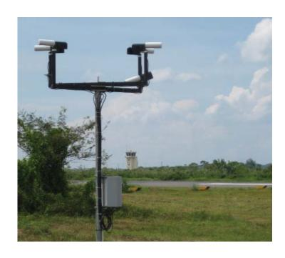
By having two direct-attenuation and two scatter values for every measurement, the 8365 Visibility Sensor does not have to depend on absolute measurements to be the most accurate sensor available today. This advantage means that measurements are independent of the effects of the environment, thereby maximizing accuracy, reducing recurring calibration, and minimizing maintenance requirements.
